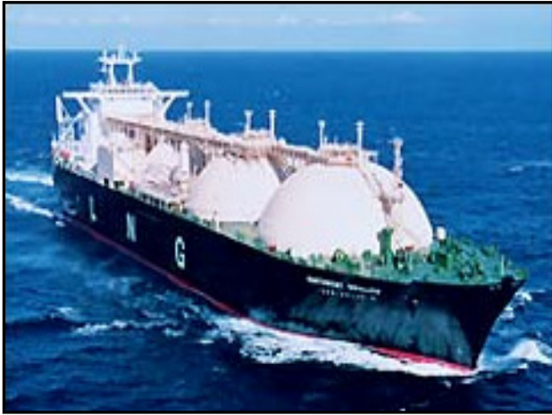
Figure 1. Example LNG carrier types (top – membrane design; below – Moss sphere design) (Source: BV 2009)
